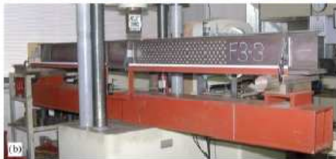
Fig. 6. Test set-up: (a) 4-point bend test; (b) 3-point bend test.
