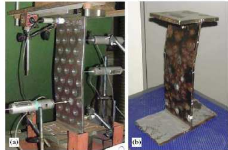
Fig. 20. Buckling behavior: (a) JE56; (b) YA.
